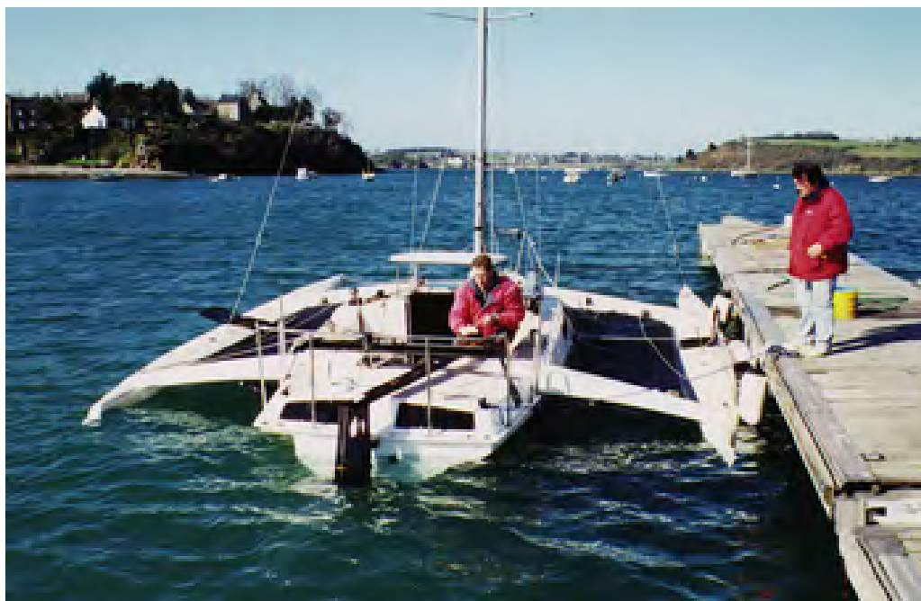
Even when fully flooded, a Farrier design will stay afloat easily. This F-27 was deliberately flooded in order to demonstrate its unsinkability.
