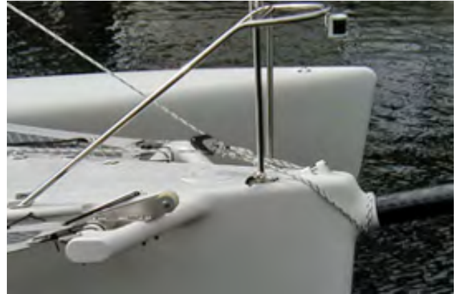
F-27 shroud tensioner - these are used to take up the slack necessary to allow easy connection of the stay to float chainplate after unfolding.
