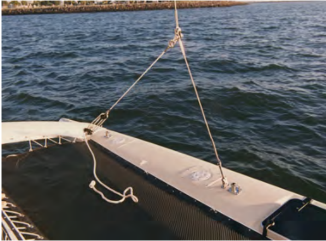
F-27 shroud tensioner - these are used to take up the slack necessary to allow easy connection of the stay to float chainplate after unfolding.
