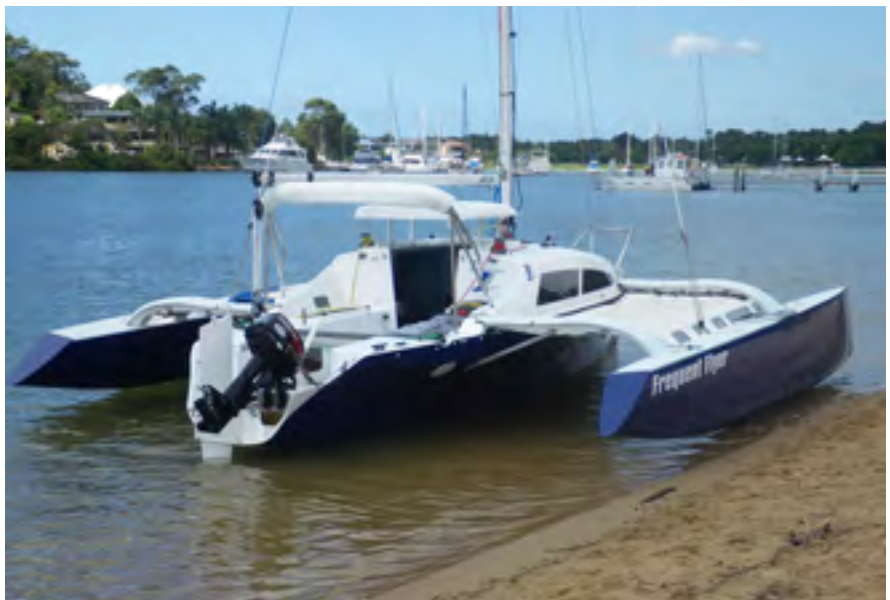
F-22 daggerboard rudder lifted partially up. The best solution for shallow water
