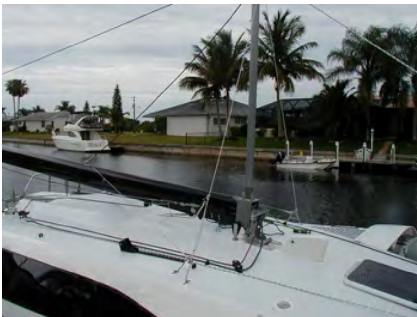
Raising wire Deck Loops - these work well to anchor raising wires as they can fold down to be flush on deck when not in use. F-33 mast step with raising pole yoke shown above and below left. The same basic mast raising setup applies for both on trailer or on water mast raising.
