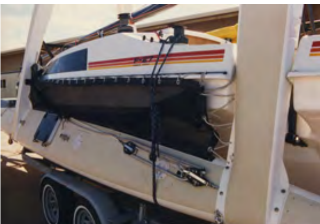
Trailer tie downs each side. Side stay tensioner can also be seen stored on float deck
