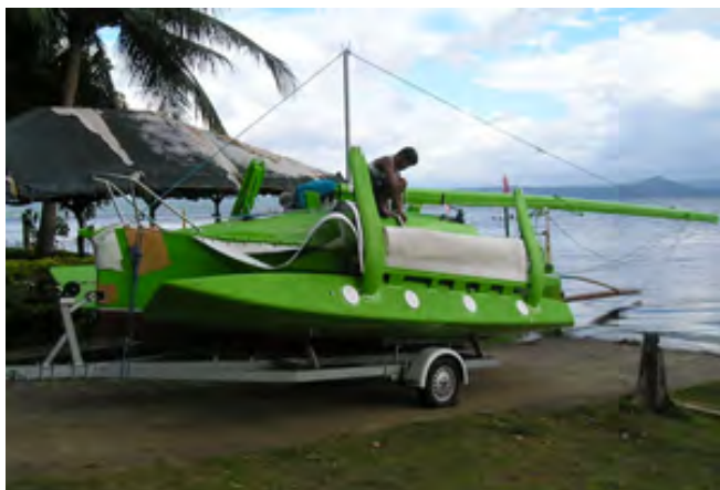
F-22 mast rolled back and attached to the deck pivot brackets, with mast raising pole in place.
