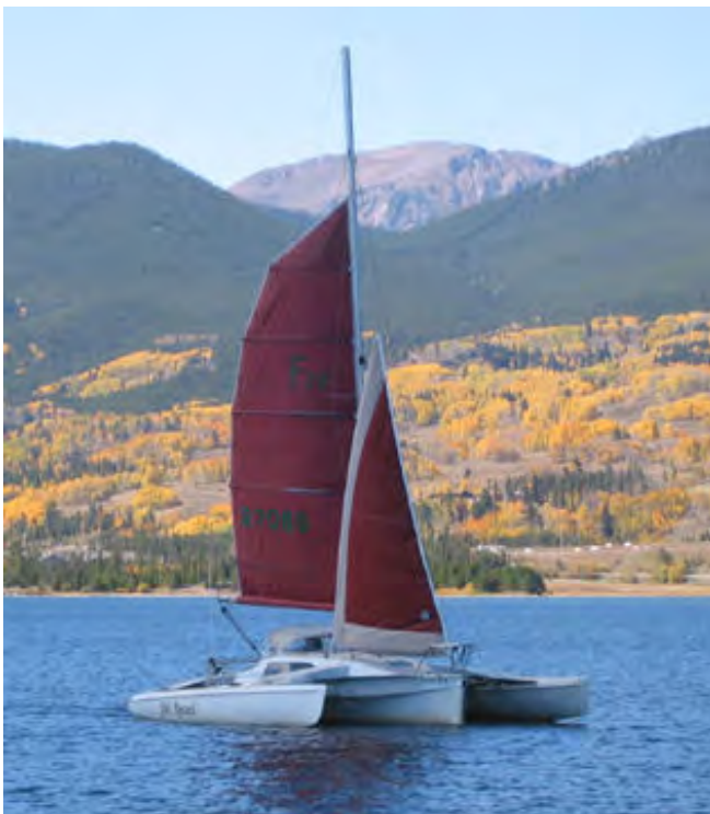
Main neatly roller reefed on an F-27
