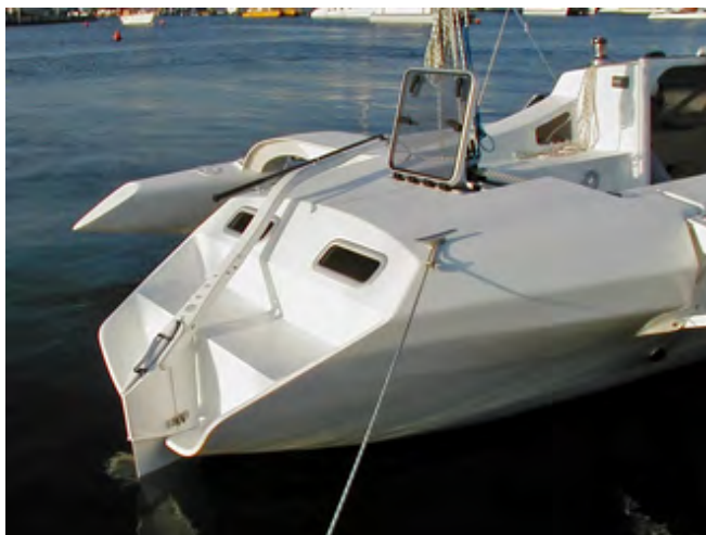
F-33 daggerboard rudder, with blade fully down
