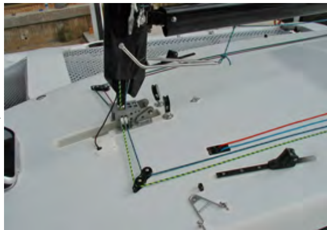
F-33 Mast Rotator Arm & attached to boom for self tacking
