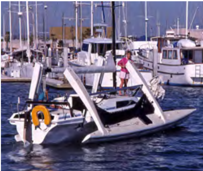
Folding can be done while motoring, but be careful in high cross winds with larger designs
