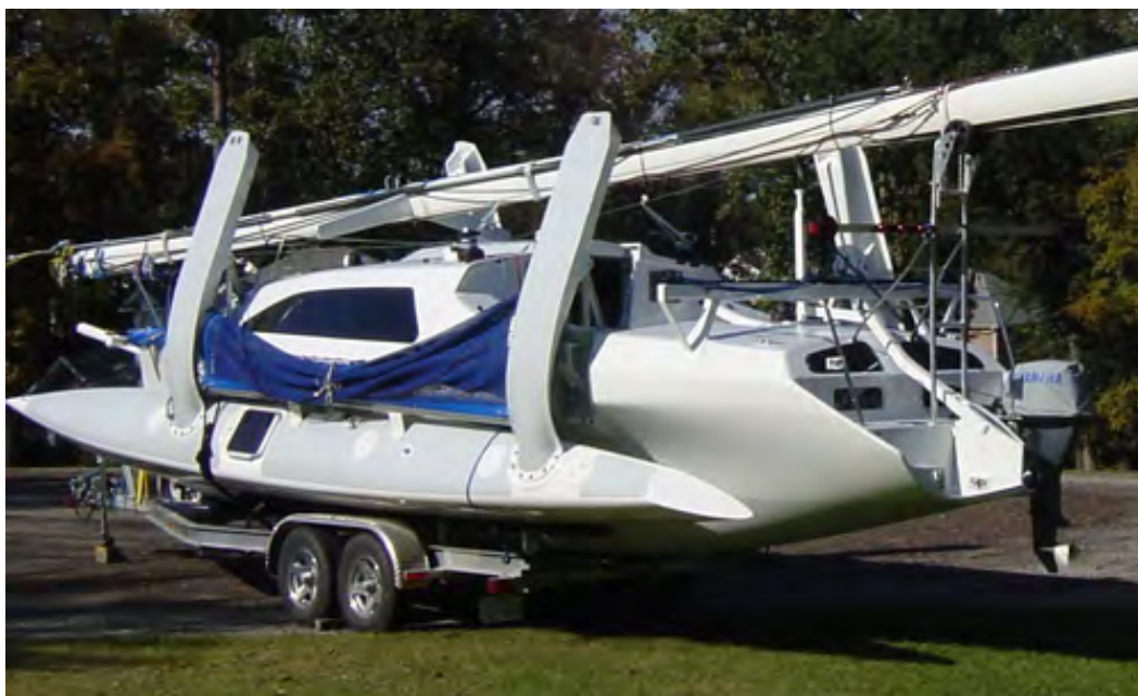
An F-33 on trailer, separate light bar in place on aft mast support, and daggerboard rudder blade removed for trailering. Lights can also be separately mounted each side (see below left), and this makes it much easier to store in vehicle.
