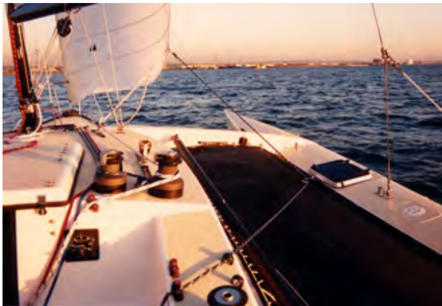
Jib barber hauler in use on an F-27 - will considerably boost performance
