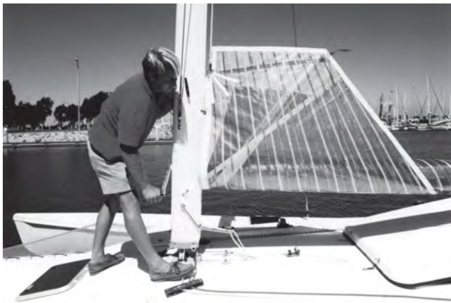
F-28 Mainsail being roller furlled. Note foot being used to control halyard.
