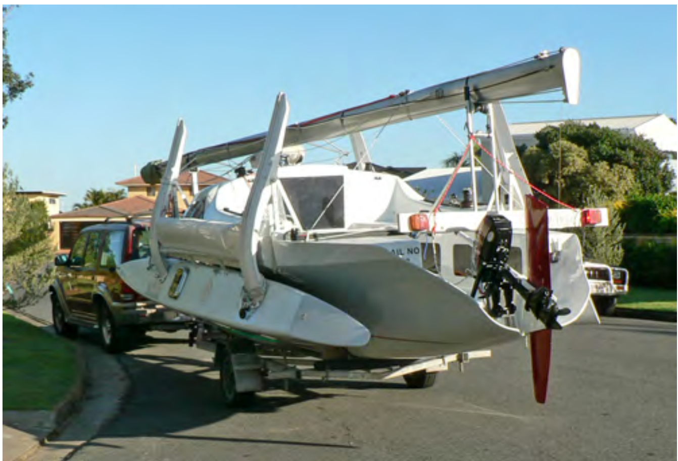
An F-22 on the trailer, with outboard and daggerboard rudder. This type of rudder can be lifted fully up for local trailering or removed altogether for long distance trips. Note separate light bar high up and well clear of water
