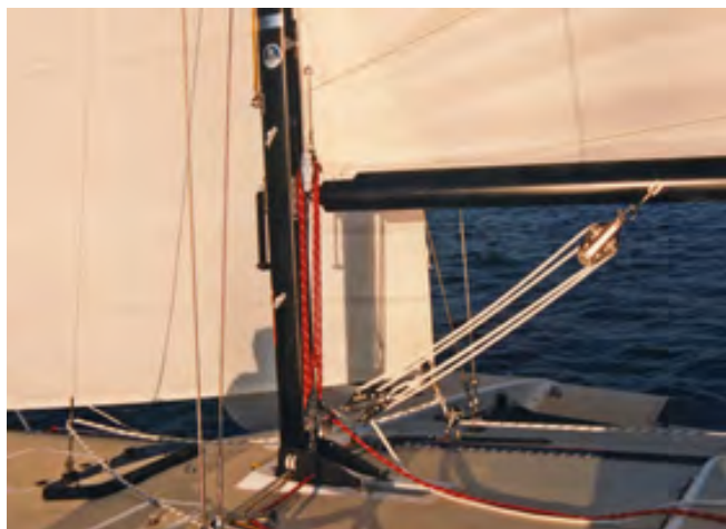
Boom vang and Cunningham eye controls on an F-27 - Boom vangs are not used with rotating masts as they will restrict rotation
